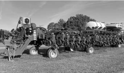
'12 Case IH 1260 36R30" planter, Precision btms., Sunco Res. Mgrs., Sunco fert. discs, PTO pump drive, AFS Pro Mon., bulk fill w/scale, planter mtd. liquid fert., in cab pneumatic down pressure.
